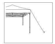
\*FRAME MUST BE SECURED DOWN TO PREVENT WIND FROM LIFTING TENT AND CAUSING DAMAGE. NOT SECURING TENT PROPERLY VOIDS THE WARRANTY.
