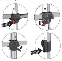
Push down lever or Push in button (method depends on the frame)
